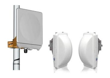
Five links are currently installed all using the unlicensed 5.4/5.8GHz frequency band from different manufacturers, with speeds ranging from 50Mbps up to 230Mbps. We believe that due to the nature of the benefits being enjoyed, the council will be considering more.
