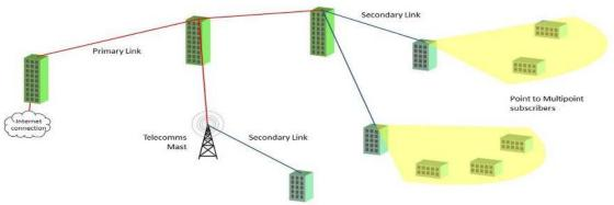
The diagram above shows a typical configuration for Metropolitan Area Network. The design is modular, allowing scaling of the network over larger areas with minimal disruption to network operations. The various elements depicted break down as follows.
